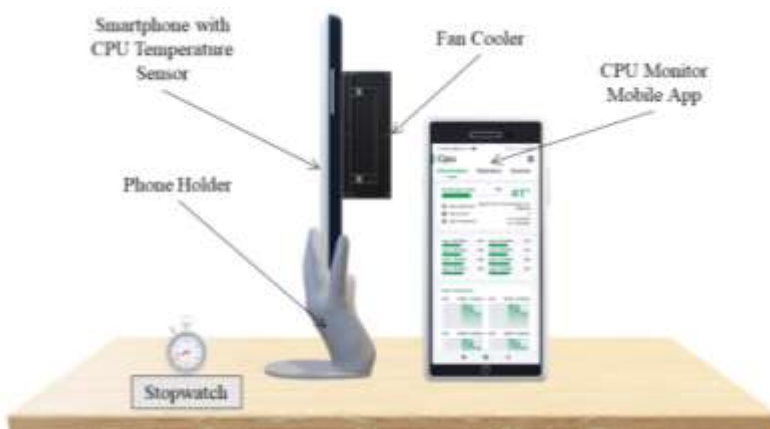
Figure 3. Setup for Experiment 2 and 3 (when the overheated phone is subjected to a fan cooler only)
